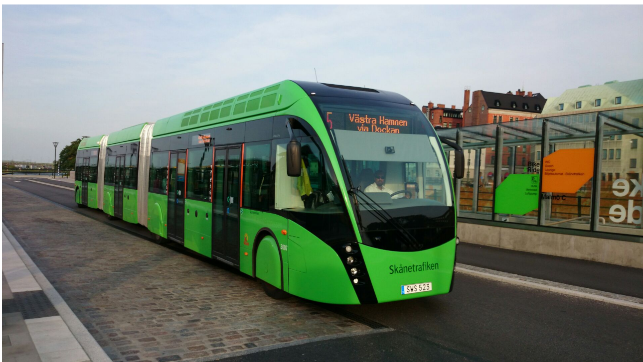
First hybrid “ tram-bus ” deployed in Malmö in June 2014. Exqui.City, manufactured by Van Hool (Belgium), are hybrid (biogas-electric) tram-buses.
